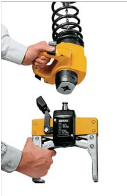
The quick-change coupling on the DSM-C control unit
