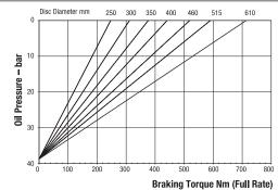
Maximum Braking Force full rate: 2.6kN Minimum Pressure for full retraction: 50 bar Weight of caliper and thruster - 5.5kg
