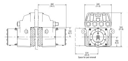
The Twiflex VMS3-SPS disc brake caliper is comprised of two modules bolted to a central mounting plate, 12mm thicker than the brake disc. Minimum disc thickness is 38mm and minimum disc diameter is 1500mm with no maximum except for practical limitations. Based on a development of the earlier Twiflex VMS2-SP disc brake, the VMS3-SPS provides a significant increase in braking force but in a similarly sized package.
