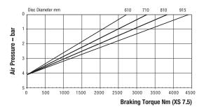
Maximum Braking Force XS 7.5: 11.2kN Minimum Pressure for full retraction: 5 bar Weight of caliper and thruster - 14.12kg Weight of thruster only - 4.9kg Volume displacement of thruster at full retraction = 1.19 l
