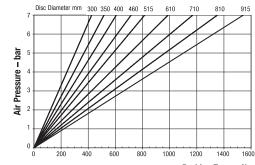
Maximum Pressure 7 bar Maximum Braking Force = 3.6kN @ 7 bar Weight of caliper and thruster - 8.15kg Braking Torque Nm Weight thruster only - 1.15kg Volume displacement of thruster at full stroke = 150ml
