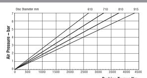
Maximum Pressure 7 bar Maximum Braking Force = 11kN @ 7 bar Weight of caliper and thruster - 11.28kg Braking Torque Nm Weight of thruster only - 2.06kg Volume displacement of thruster at full stroke = 426ml
