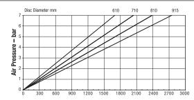
Maximum Pressure 7 bar Maximum Braking Force = 6.9kN @ 7 bar Weight of caliper and thruster - 10.54kg Braking Torque Nm Weight of thruster only - 1.32kg Volume displacement of thruster at full stroke = 300ml
