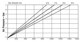
Maximum Pressure 7 bar Maximum Braking Force = 3.6kN @ 7 bar Weight of caliper and thruster - 10.37kg **Braking Torque Nm**Weight of thruster only - 1.15kg
