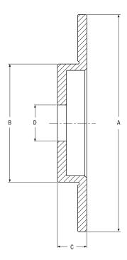
Twiflex brake discs may be supplied bored and drilled to customer requirements. Non-standard disc sizes, not shown in the tables, can be supplied to order. Brake discs are manufactured from spheroidal graphite iron.
