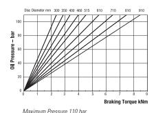
Maximum Prasking Force = 20kN @ 110 bar Weight of caliper - 5.82kg Volume displacement per 1mm stroke at each pad = 4.8ml
