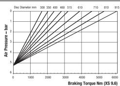
Minimum Pressure for full retraction: 6.4 bar Maximum Braking Force XS 9.6: 14.3kN Weight of caliper and thruster - 12.1kg Weight of thruster only - 5.1kg Volume displacement of thruster at full retraction = 1.19 l
