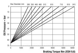
Minimum Pressure for full retraction: 82 bar Maximum Braking Force XSH 9.6: 14.3kN Weight of caliper and thruster - 11.6kg Weight of thruster only - 4.6kg Volume displacement of thruster at 6mm retraction = 9.1ml
