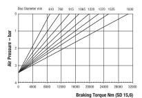
Maximum Braking Force SD 15.6: 36kN Minimum Pressure for full retraction: 4.6 bar Weight of caliper and thruster - 55kg Weight of thruster only - 21kg Volume displacement of thruster at full retraction = 2.5 l
