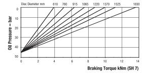
Maximum Braking Force SH 7: 16.5kN Minimum Pressure for full retraction: 59 bar Weight of caliper and thruster - 49.7kg Weight of thruster only - 15.7kg Volume displacement of thruster at full retraction = 56ml
