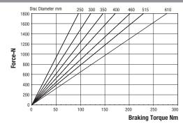
Maximum Braking Force = 1.01kN Weight of caliper and hand wheel assembly - 2.53kg Weight of hand wheel assembly only - 1.03kg
