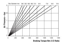
Minimum Pressure for full retraction: 2.5 bar Maximum Braking Force 1/2 rate: 3.2kN Weight of caliper and thruster - 10.5kg
