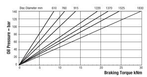
Maximum Pressure 140 bar Maximum Braking Force = 36kN @ 140 bar Weight of caliper and thruster - 36.9kg Weight of thruster only - 2.9kg Volume displacement of thruster at full stroke = 40ml
