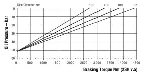
Maximum Braking Force XSH 7.5: 11.2kN Minimum Pressure for full retraction: 63 bat Weight of caliper and thruster - 13.62kg Weight of thruster only - 4.4kg Volume displacement of thruster at 6mm retraction = 9.1ml
