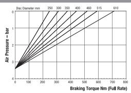
Maximum Braking Force full rate: 2.6kN Minimum Pressure for full retraction: 5 bar Weight of caliper and thruster - 4.9kg
