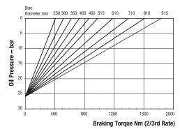
Minimum Pressure for full retraction 33 bar Maximum Braking Force 2/3rd rate: 4.3kN Weight of MR caliper and thruster - 10.5kg Weight of MR2 caliper and thruster - 11kg Weight of thruster only - 4kg Volume displacement of thruster at 4mm retraction = 5ml
