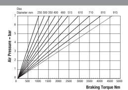
Maximum Pressure 7 bar Maximum Braking Force = 10.8kN @ 7 bar Weight of MR caliper and thruster - 8.56kg Weight of MR2 caliper and thruster - 9.06kg Weight of thruster only - 2.06kg Volume displacement of thruster at full stroke = 426ml
