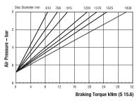
Maximum Braking Force S 15.6: 36kN Minimum Pressure for full retraction: 8.4 bar Weight of caliper and thruster - 49kg Weight of thruster only - 15kg Volume displacement of thruster at full retraction = 1.3 l
