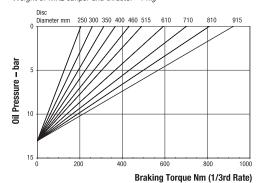
Minimum Pressure for full retraction: 17 bar Maximum Braking Force 1/3rd rate: 2.2kN Weight of MR caliper and thruster - 10.5kg Weight of MR2 caliper and thruster - 11kg Weight of thruster only - 4kg Volume displacement of thruster at 4mm retraction = 5ml
