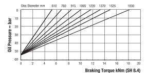
Maximum Braking Force SH 8.4: 19.5kN Minimum Pressure for full retraction: 65 bar Weight of caliper and thruster - 50.2kg Weight of thruster only - 16.2kg Volume displacement of thruster at full retraction = 56ml
