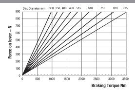
Weight of caliper and lever assembly - 8.4kg Weight of lever assembly only - 1.4kg Maximum Braking Force = 8.3kN @ 0.9kN force on lever
