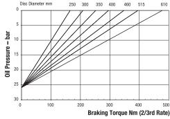
Maximum Braking Force 2/3rd rate: 1.74kN Minimum Pressure for full retraction: 33 bar Weight of caliper and thruster - 5.5kg
