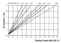
Maximum Braking Force SD 11: 25kN Minimum Pressure for full retraction: 3.3 bar Weight of caliper and thruster - 53.2kg Weight of thruster only - 19.2kg Volume displacement of thruster at full retraction = 2.5 l
