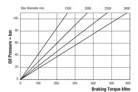
Maximum Pressure 110 bar Maximum Braking Force = 433kN @ 110 bar Weight of caliper (2 modules ) - 580kg Volume displacement per 1mm stroke at both pads = 101.5ml
