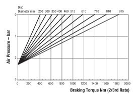
Minimum Pressure for full retraction: 3.3 bar Maximum Braking Force 2/3rd rate: 4.3kN Weight of MR caliper and thruster - 10.0kg Weight of MR2 caliper and thruster - 10.5kg Weight of thruster only - 3.5kg Volume displacement of thruster at full retraction is 950ml
