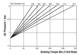
Maximum Braking Force 1/3rd rate: 0.87kN Minimum Pressure for full retraction: 1.7 bar Weight of caliper and thruster - 4.9kg
