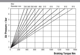
Maximum Pressure 7 bar Maximum Braking Force = 3.5kN @ 7 bar Weight of MR caliper and thruster - 7.65kg Weight of MR2 caliper and thruster - 8.15kg Weight thruster only - 1.15kg Volume displacement of thruster at full stroke = 150ml
