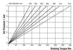
Maximum Pressure 7 bar Maximum Braking Force = 1.44kN @ 7 bar Weight of caliper and thruster - 2.5kg Weight thruster only - 1.0g
