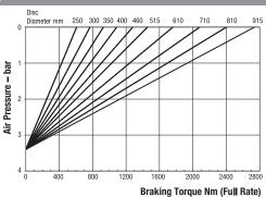
Minimum Pressure for full retraction: 5 bar Maximum Braking Force full rate: 6.4kN Weight of MR caliper and thruster - 10.0kg Weight of MR2 caliper and thruster - 10.5kg Weight of thruster only - 3.5kg Volume displacement of thruster at full retraction is 950ml
