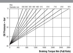
Minimum Pressure for full retraction: 50 bar Maximum Braking Force full rate: 6.4kN Weight of MR caliper and thruster - 10.5kg Weight of MR2 caliper and thruster - 11kg Weight of thruster only - 4kg Volume displacement of thruster at 4mm retraction = 5ml
