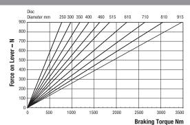
Weight of MR caliper and thruster - 7.9kg Weight of MR2 caliper and thruster - 8.4kg Weight of lever assembly only - 1.4kg Maximum Braking Force = 8.3kN @ 0.9kN force on lever
