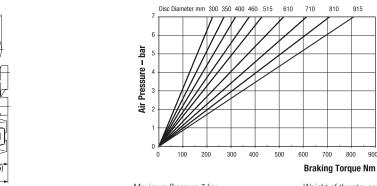
Maximum Pressure 7 bar Maximum Braking Force = 1.9kN @ 7 bar Weight of caliper and thruster - 7.3kg
