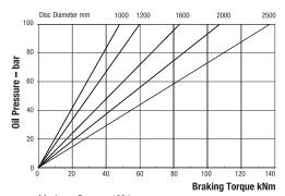
Maximum Pressure 100 bar Maximum Braking Force = 118kN @ 100 bar Weight of caliper (2 modules) - 80kg Volume displacement per 1mm stroke at both pads = 31ml
