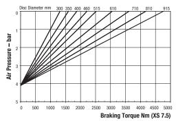
Minimum Pressure for full retraction: 5.5 bar Maximum Braking Force XS 7.5: 11.2kN Weight of caliper and thruster - 11.9kg Weight of thruster only - 4.9kg Volume displacement of thruster at full retraction = 1.19 l
