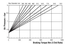
Minimum Pressure for full retraction: 1.7 bar Maximum Braking Force 1/3 rate: 2.2kN Weight of caliper and thruster - 10.5kg
