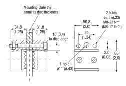
The Twiflex T2 disc brake caliper is split caliper design suitable for use with a minimum disc thickness of 5mm. The modules are mounted each side of a central mounting plate of the same thickness as the brake disc. Minimum disc diameter is 120mm. Alternatively, the brake may be side-mounted with a spacer equal to the disc thickness between the two halves.
