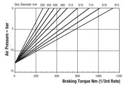
Minimum Pressure for full retraction: 17 bar Maximum Braking Force 1/3rd rate: 2.2kN Weight of caliper and thruster - 11kg
