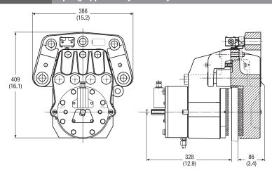
The Twiflex VKSD-FL disc brake caliper comprises a single spring module forming the 'active' side of this floating unit and is available for use where space is limited or to accommodate axial disc float of  $\pm 6$ mm.
