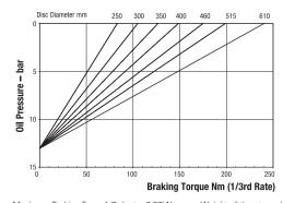
Maximum Braking Force 1/3rd rate: 0.87kN Minimum Pressure for full retraction: 17 bar Weight of caliper and thruster - 5.5kg
