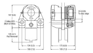
The Twiflex T40 disc brake caliper is split caliper design suitable for use with a minimum disc thickness of 20mm. The modules are mounted each side of a central mounting plate of the same thickness as the brake disc. Minimum disc diameter is 300mm.
