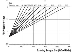
Minimum Pressure for full retraction: 1.7 bar Maximum Braking Force 1/3rd rate: 2.2kN Weight of MR caliper and thruster - 10.0kg Weight of MR2 caliper and thruster - 10.5kg Weight of thruster only - 3.5kg Volume displacement of thruster at full retraction is 950ml
