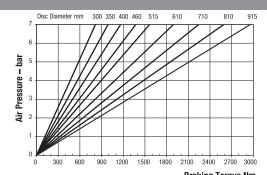
Maximum Pressure 7 bar Maximum Braking Force = 6.9kN @ 7 bar Weight of caliper and thruster - 8.32kg **Braking Torque Nm**Weight of thruster only - 1.32kg
