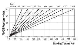
Maximum Pressure 20 bar Maximum Braking Force = 2kN @ 20 bar oil or air pressure Weight of caliper - 0.75kg Volume displacement per 1mm stroke at each pad = 3ml
