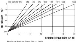
Maximum Braking Force SH 15: 35kN Minimum Pressure for full retraction: 120 bar Weight of caliper and thruster - 53kg Weight of thruster only - 19kg Volume displacement of thruster at full retraction = 56ml
