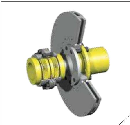
The **SDF** Coupling is a Double Engagement Gear Coupling manufactured with two flanged sleeves with internal spur gear teeth, connected with a set of heat treated alloy steel fasteners and meshed with accurately matched, machined and ground crown toothed hubs.
